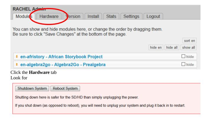
To Shutdown simply click the **Shutdown System** button, wait until the activity light on the Pi stops, I usually give it 10 to 15 seconds, then pull the power cable out.
