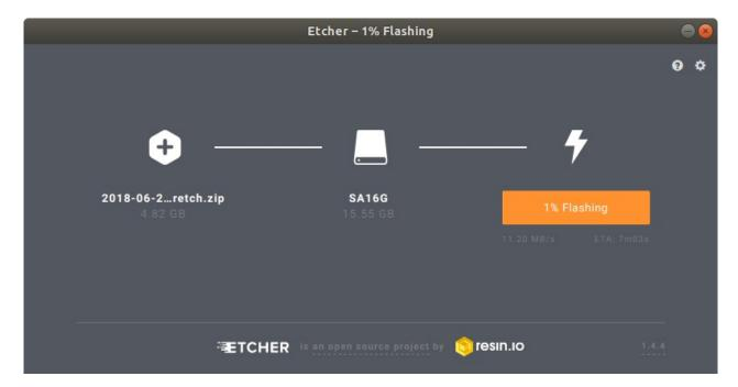
Once the SD card is ready, eject it and insert in your Raspberry Pi
