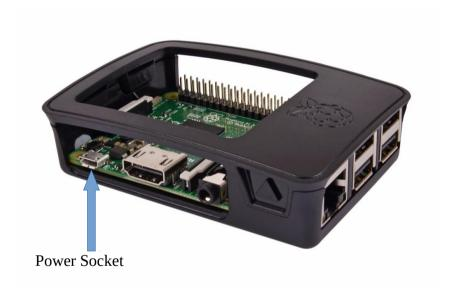
Once connected the Raspberry Pi will automatically set itself as a WiFi access point. Its SSID (or WiFi name ) is Rpi. Any wireless device, a laptop, tablet, phone or even a PC with wireless capability can connect to this (without the need for a password)
